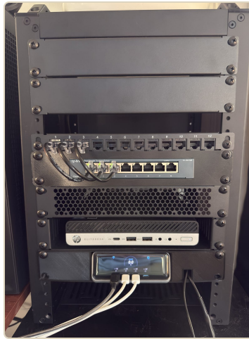
special-k, the HP EliteDesk Mini that runs the whole homelab, mounted in a 10-inch rack under the patch panel and switch.
