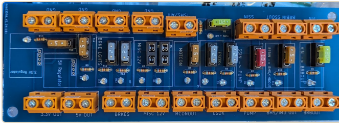
The populated fusebox. One fuse and one indicator LED per circuit, with the shutdown-circuit signals labeled on the silkscreen.
